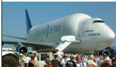
I attached a picture of the Boeing Dreamliner. This is a modified 747-400 used to ferry parts for the new 787 Dreamliner. 3 dreamliners are currently in use with a 4th being modified. The tail swings
